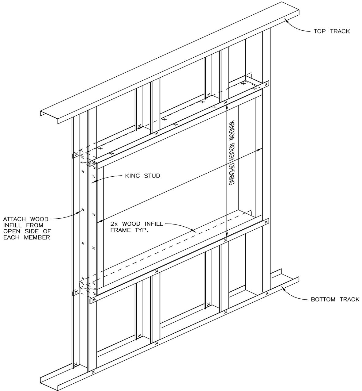
Figure C7.2.2 Window Framing Detail - 2
