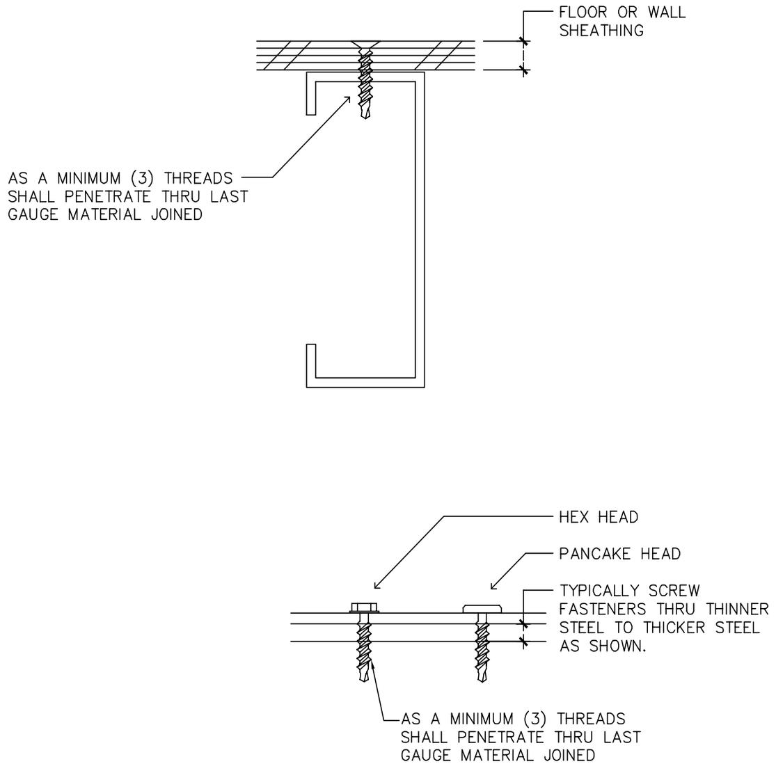
Figure C2.11 Screw Attachments
